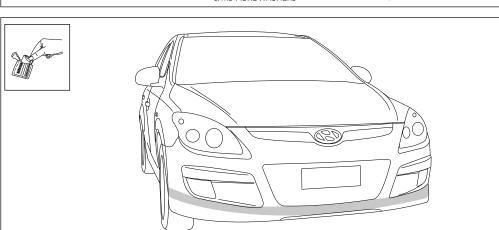
**4.**Clean the shaded areas using the alcohol wipes provided and wipe away residue with a dry clean cloth.
